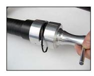
6. Remove the tool guide and repeat the jacket stripping operation (step 2).
