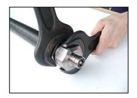
11. Then tighten to mechanical stop by the use of two spanners. Tighten by rotating the back nut while holding the front nut stationary.
