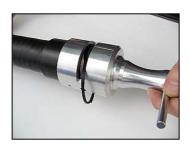
2. Strip the jacket using the jacket tool. Press and turn against the cable until the mechanical stop is reached.
