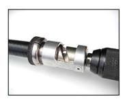
5. - and strip the cable. Press against the cable and turn slowly (app. 300 rpm) until the physical stop is reached.
