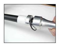
2. Strip the jacket using the jacket tool. Press and turn until the mechanical stop is reached.
