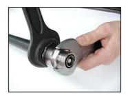
11. Then tighten to mechanical stop by the use of two spanners. Tighten by rotating the back nut while holding the front nut stationary.
