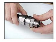
10. Click the front part against the cable and screw the back nut against the front as far as possible by hand.
