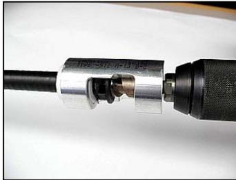
1. Cut your cable and strip it with the stripping tool as shown.
