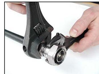
9. Then tighten to mechanical stop by the use of two spanners. Retain the front part in the same position during this operation.
