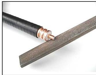
5. Chamfer the center conductor.
