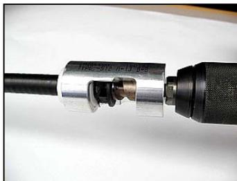
4. Repeat the stripping operation. Press against the cable and turn slowly (app. 300 rpm) until the physical stop is reached.
