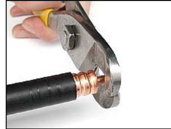
3. If not, cut a small piece of the center conductor corresponding to the "missing" length to the top of a curve.
