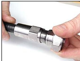
8. "Click" the front part on the cable and screw the back nut against the front as far as possible by hand.
